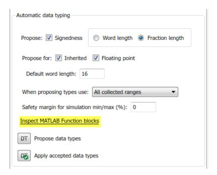
The window that opens helps you to inspect advanced conversion settings such as fimath settings, and MATLAB function replacements.
